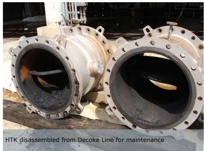
HTK disassembled from Decoke Line for maintenance
