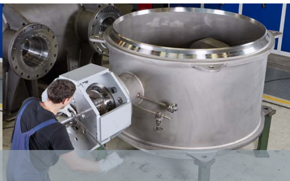
4. The shaft is mounted and gets tightened with the help of bolts in the flange.
