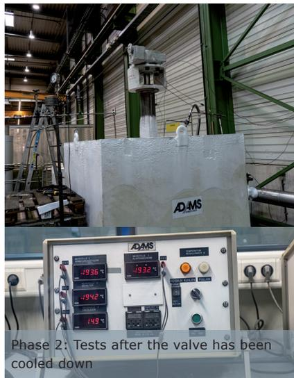
Phase 2: Tests after the valve has been cooled down
