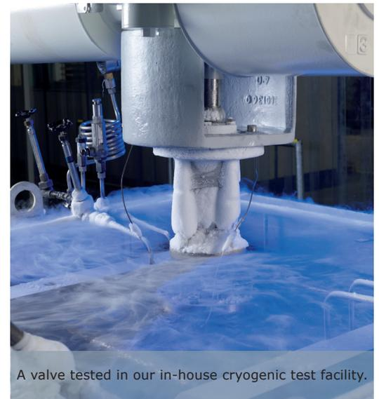
A valve tested in our in-house cryogenic test facility.
