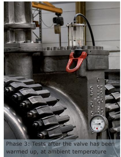
Phase 3: Tests after the valve has been warmed up, at ambient temperature
