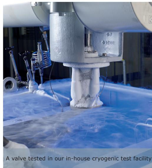
A valve tested in our in-house cryogenic test facility.
