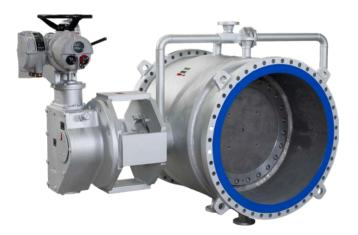
The HTK valve is a rotary tight shut-off valve with metal-to-metal seat for use at high temperatures. A number of small purging holes equally spaced on the seat in a single row (DV) or in double rows (TLV) provide continuous steam purging of the seat to prevent coke build-up on the seating surface. A patented disc seal protection device (Flow Deflector) prevents disc edge erosion caused by coke particles in the flow stream in the full open position.
